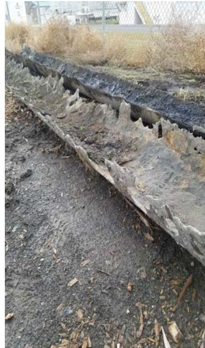
seeing extensive corrosion but the first 20-30 feet of ductile iron pipe was rotted away. While this didn't happen overnight, we wanted to share it with Council so you can see some of the challenges we face and how it can impact infrastructure. This was a line we planned to replace with the treatment plant upgrades. Due to the delay caused by the TMDL rules, the pipe had other plans. You can see that the pipe rotted into two pieces. Additionally, you can see the corrosion on the
